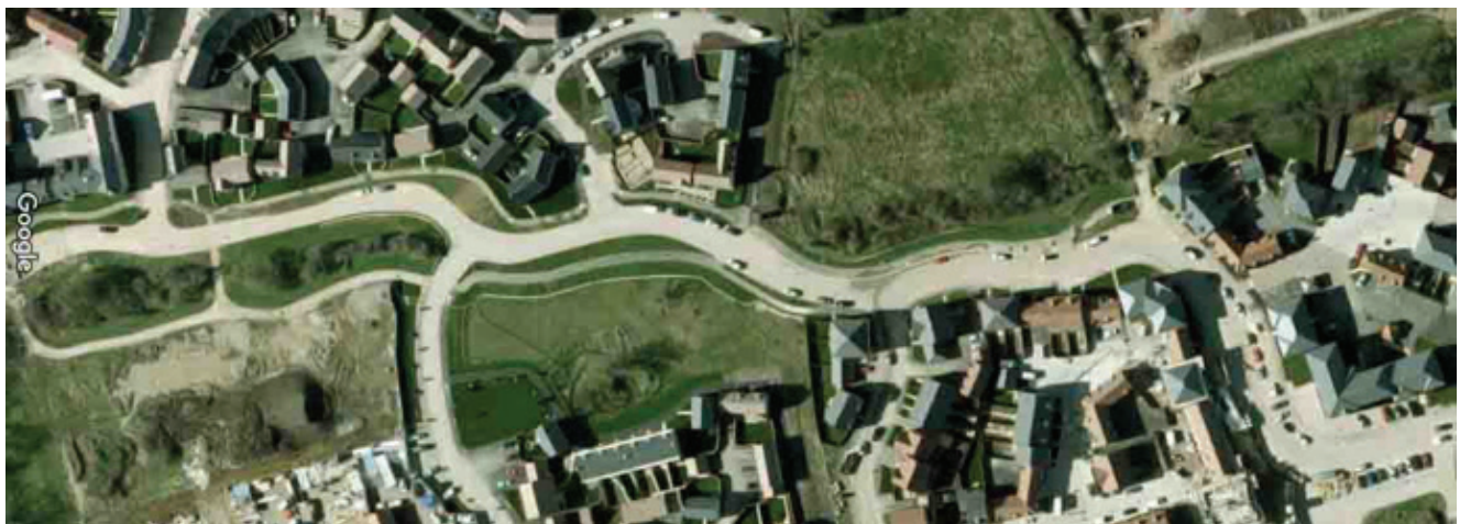
Figure 17: Poor urban design: gratuitous curves on a bus route bring no benefits (a town in southern England). (Image by Google)
